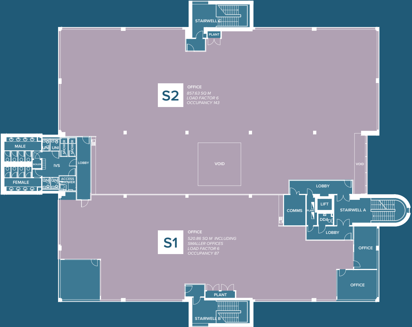
SECOND FLOOR GENERAL ARRANGEMENT
